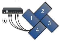
2. Connect the input source to the controller's input.
