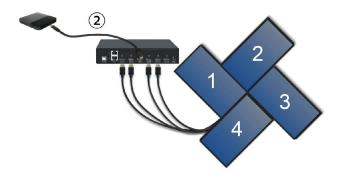
3. Connect a PC with the installed control software to the controller's USB port.
