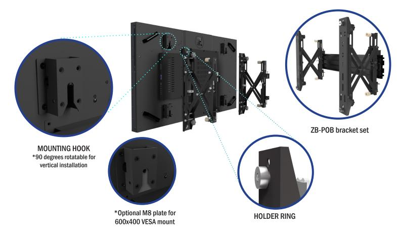
HH-Series Displays have four Mounting Hooks at the 600x400mm VESA position for Hanging onto the four holder rings that are attached to the mounting bracket. The mounting bracket can be the ZDS Pushout Bracket, or any mounting bracket of your choice.
